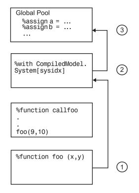
**File Scope.** File scopes are searched before the global scope, as shown in the following diagram.
