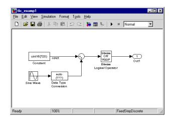
The code generated for the bit-wise operator block reuses a temporary variable that is set up for the output of the sum block to save memory. This results in one very efficient line of code, as seen here.
