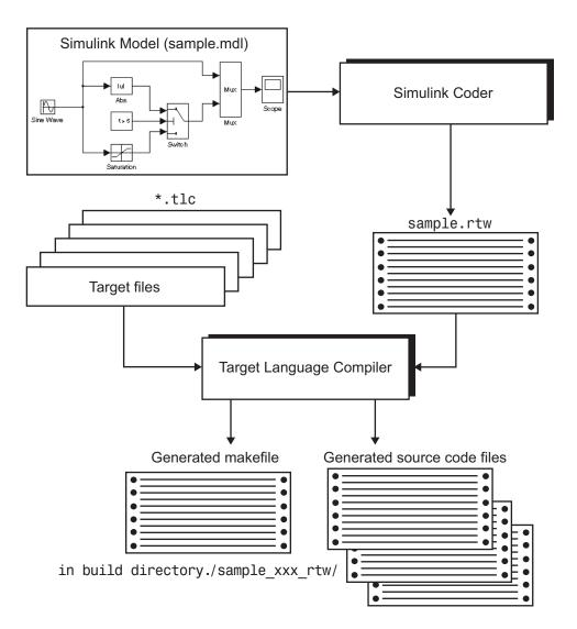
When generating code from a Simulink model, the first step in the automated process is to generate a *model*.rtw file. The *model*.rtw file includes all the model-specific information required for generating code from the Simulink model. *model*.rtw is passed to the Target Language Compiler, which uses it in combination with a set of included system target files and block target files to generate the code.
